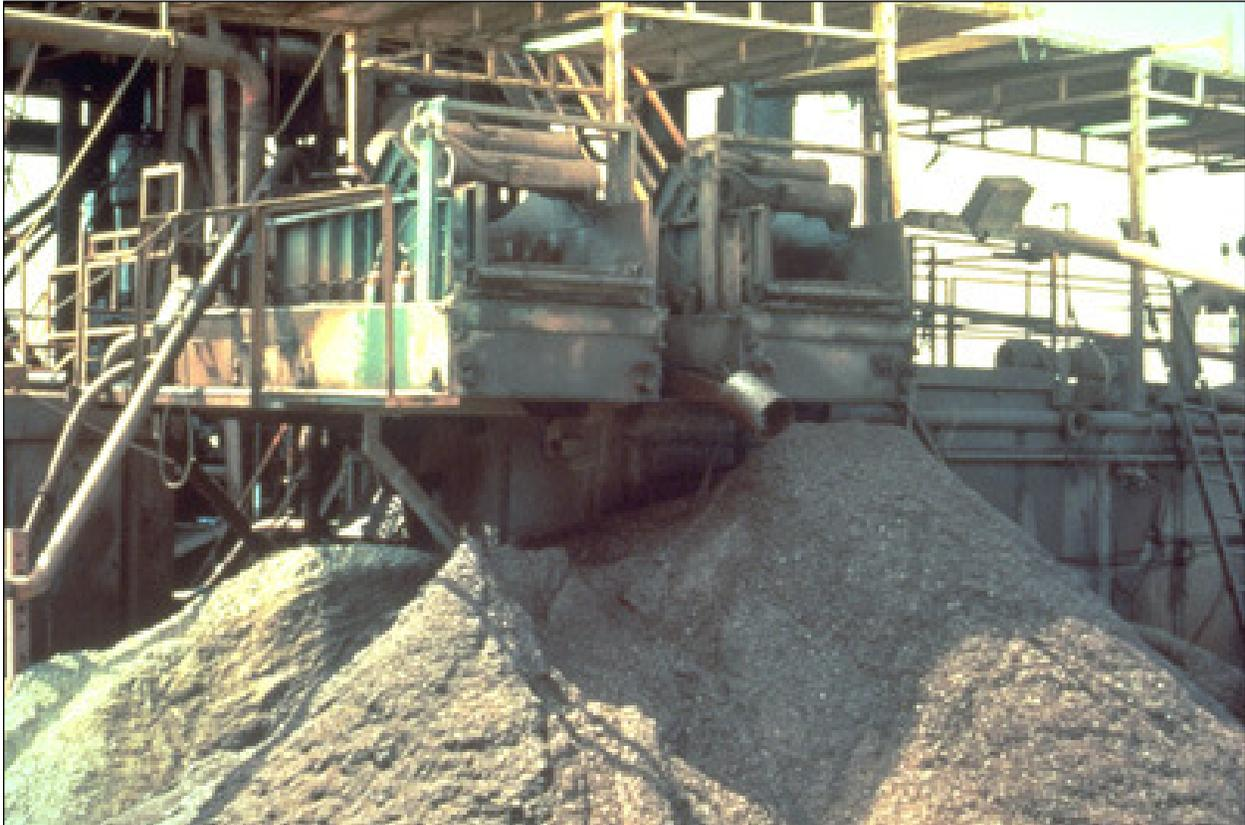
**Figure 6. Rock cutting shakers**
