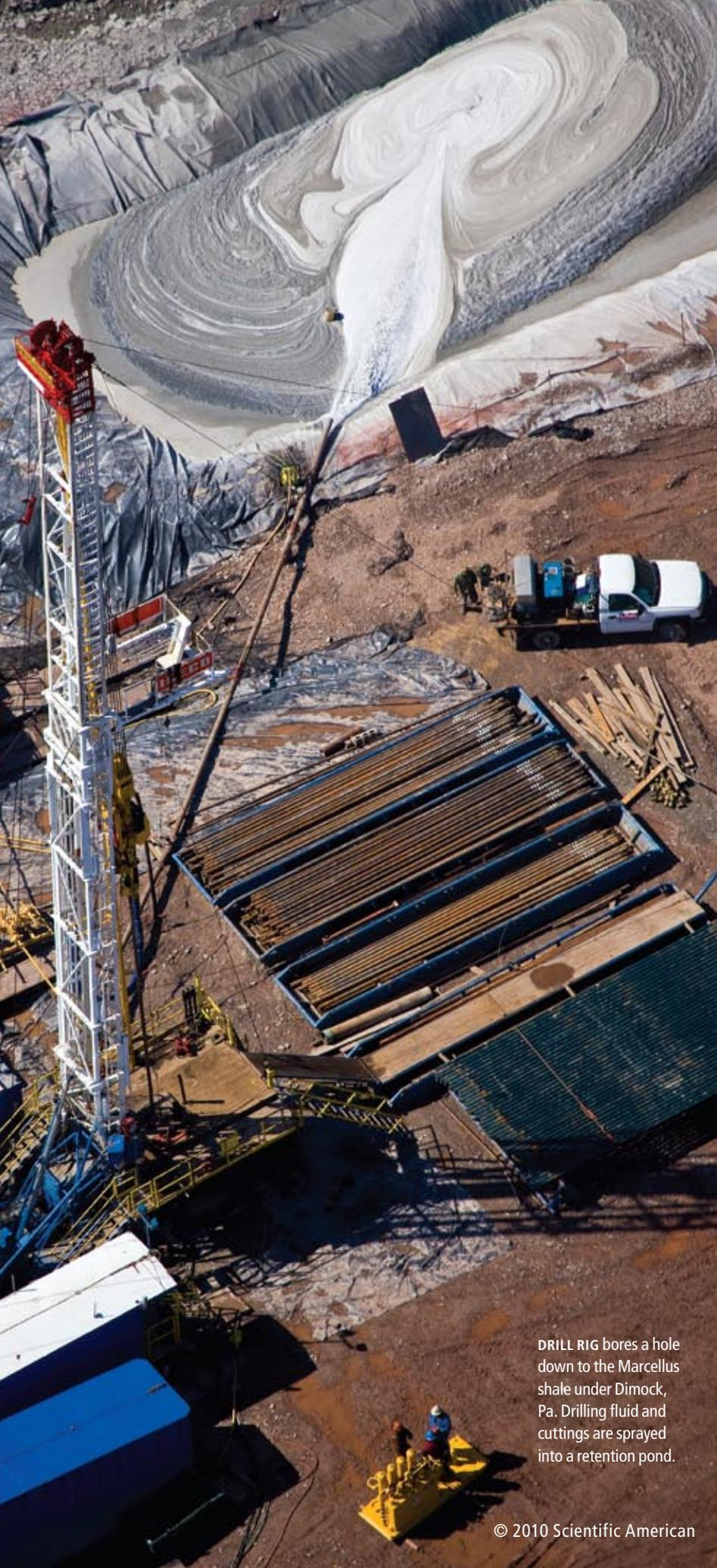
DRILL RIG bores a hole down to the Marcellus shale under Dimock, Pa. Drilling fluid and cuttings are sprayed into a retention pond.
