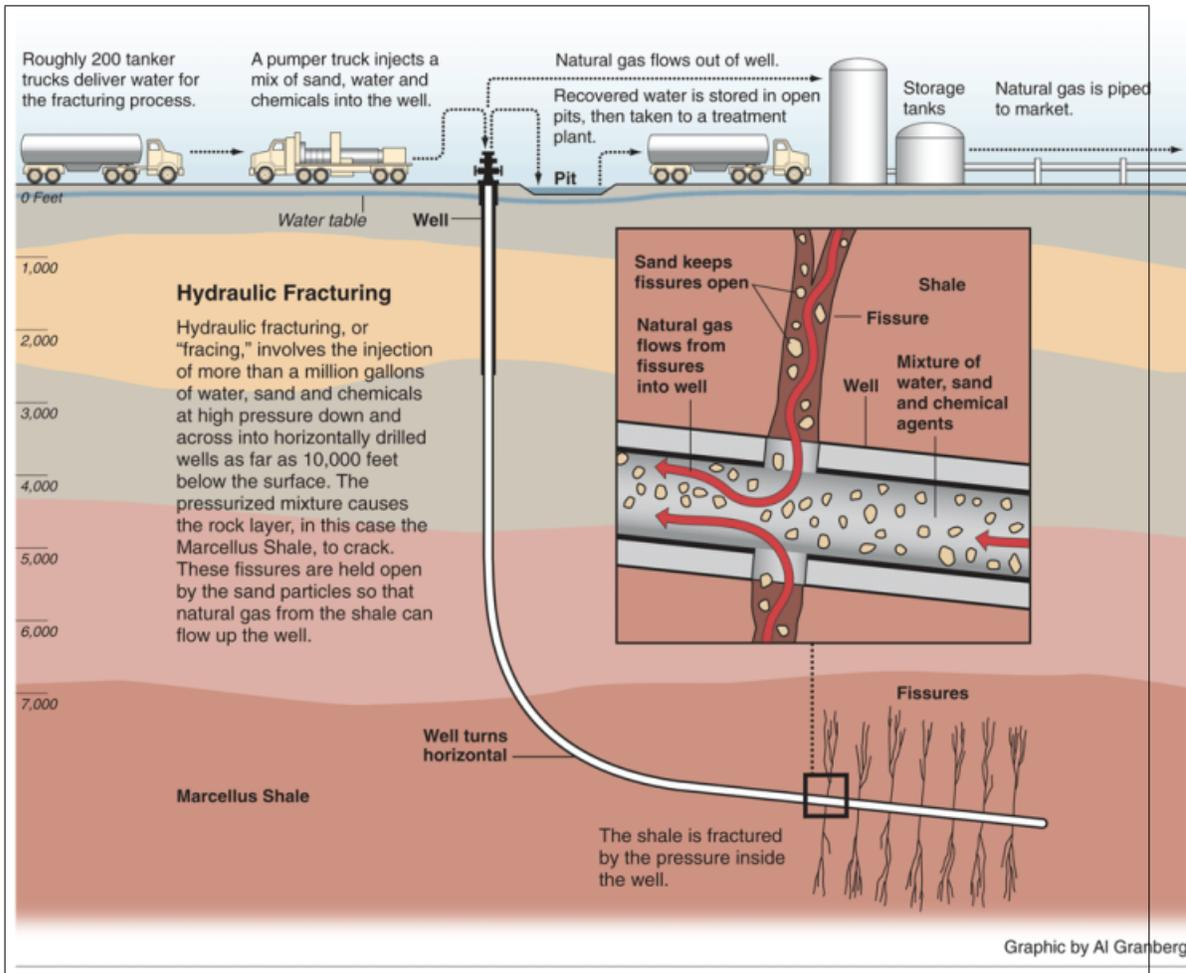
Figure 1: Graphical Representation of NGD Process
